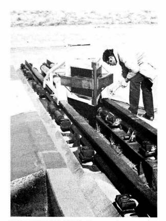
DAVE PRESTON (1525), test engineer, makes final check of rocket sled before launch. Nose of the sled changed angle of attack during the run from 20 degrees at launch to zero degrees at the end of the test.
